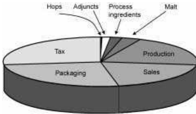
Fig. 1.1 A generalised breakdown of major costs associated with the brewing of beer.
