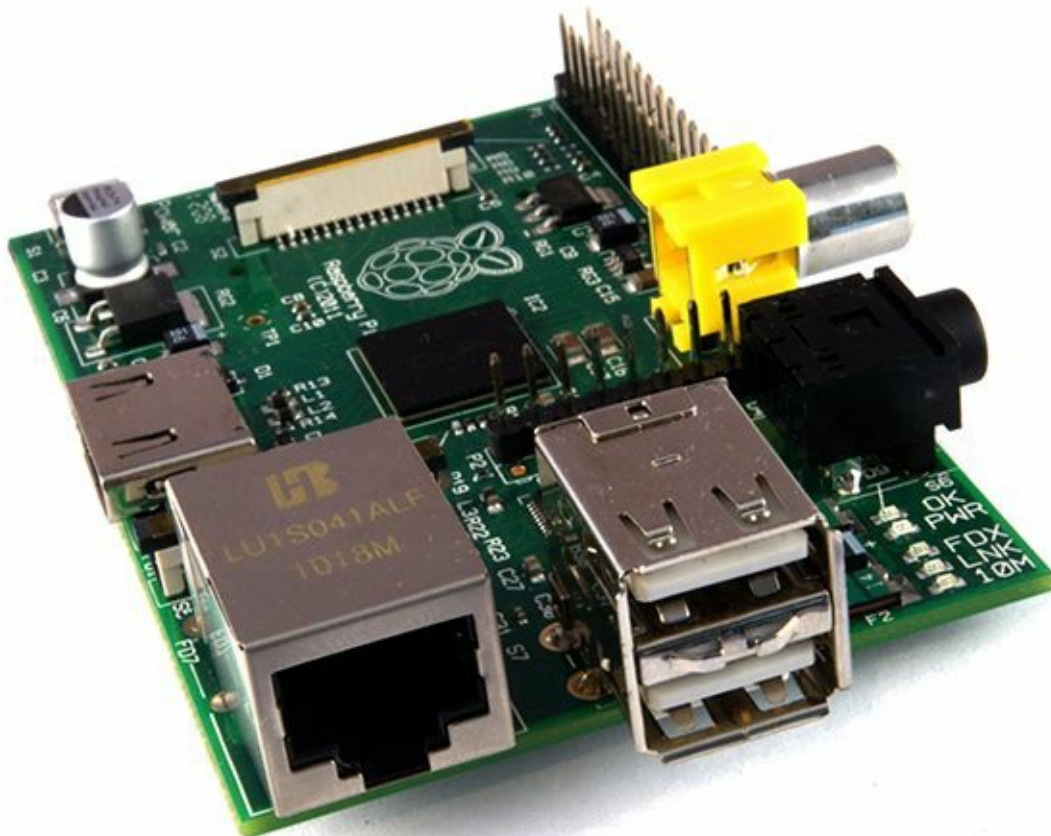
Figure 1-4: Model B's two USB ports
